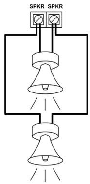
Two 8 Ohm Speakers in Series, One in Parallel (6 ohm load)
